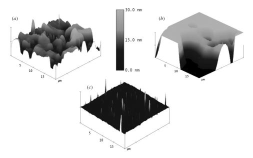
Figure 6. AFM images of a polymeric film (AG I) on Si substrates for three deposition: (a) 30 s, (b) 240 s, and (c) 300 s.
