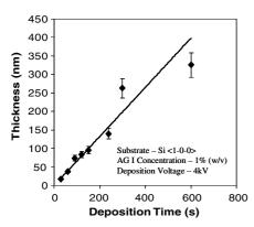
**Figure 4.** Thickness versus deposition time of a polymeric film (AG I) on Si substrates.
